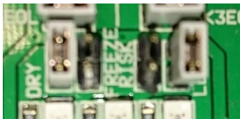
Jumper positions for DRY PIPE (Output 3) and SUB-ALARM FLOW EVENT(Output 4)
