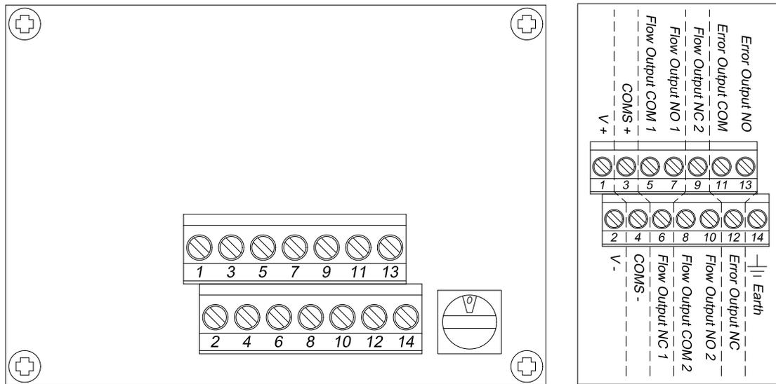
Before installing the unit the flow signal delay timer can be set. Remove the top lid and locate the rotary position switch mounted on the PCB. Setting '0' will select the minimum delay and setting '9' the maximum delay. Settings between these will set the delay proportionally. The factory set default position is 9.
